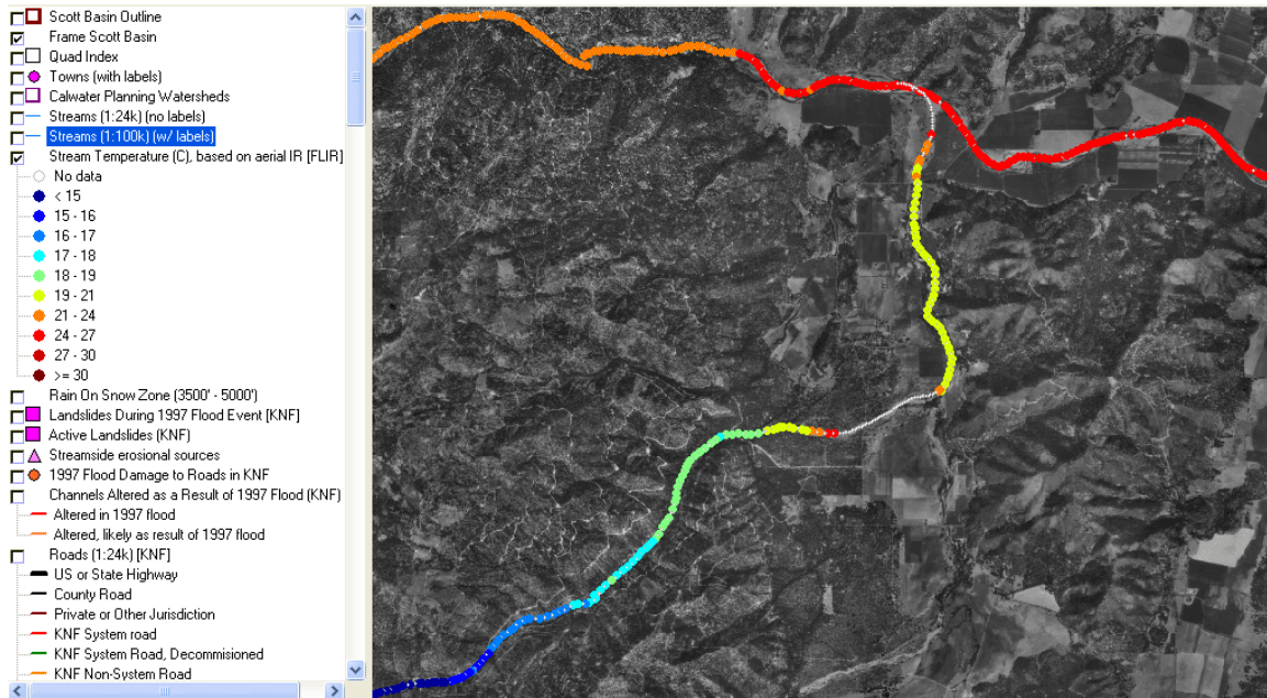
Figure 19. This map shows summary data of Scott River Thermal Infrared Radar (TIR) surveys for Shackleford Creek. Shackleford Creek flows northeast, then north to meet up with the mainstem Scott at the top of the figure. Note that temperature increases as flow is depleted. Missing temperatures (shown as grey reaches) indicates the stream is dry.
